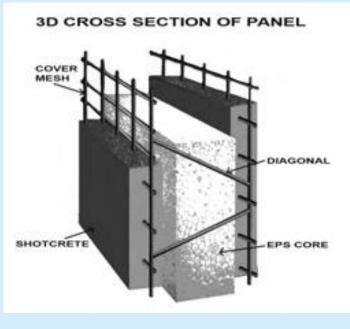
angle for superior strength and welded to each of the outer layer sheet of steel welded wire fabric mesh. The panels are finished at the site using minimum 30 mm thick shotcrete of cement & coarse sand in the ratio of 1:4 applied under pressure.(Refer sectional details as shown). The shotcrete coat encases the EPS Core with centrally placed streel welded wire fabric mesh.
